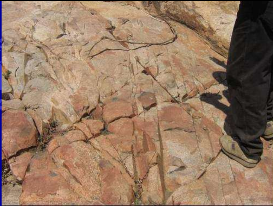
Right bank river section 200m downstream of center line, gneissic granite intersected by 4 joint sets.
